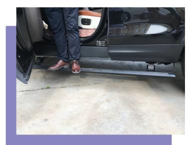
The  $VERSA^{SUV}$  is an electrically operated double sided swing out step. The step has been designed specifically for SUV vehicles and covers the full side of the vehicle providing a step for both the front and the rear door.
